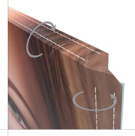
Insert the 90° positioned textile starting at the corners.
