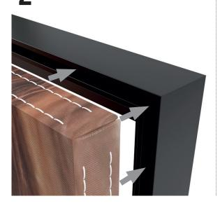
Once all the corners are placed, slip your finger along the rubber stripe until it is smartly fit into the frame.
